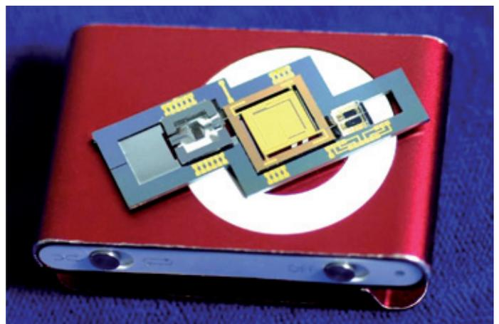
▲ A 25 cm separation column of a palm-size  $\mu$ GC with embedded thermal sensing and closed-loop microprocessor-based control on a 2nd. Generation Apple iPod Shuffle (K. Wise, Univ. Michigan)
