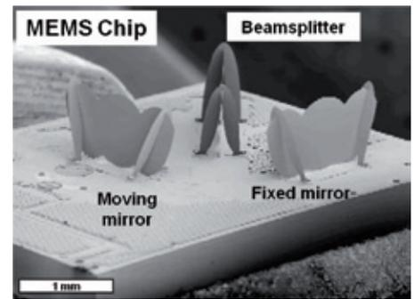
▲ MEMS-chip with spectrometer parts (fixed and moving mirror, beam splitter) on a data processing chip (Block Chem Pen)
